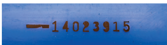
Shift code for a PE100 pipe
